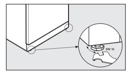
■ To align the appliance, adjust the feet using the spanner supplied.
